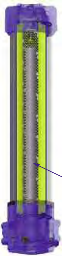
P02 "Internal tube for reduced flow rates"
